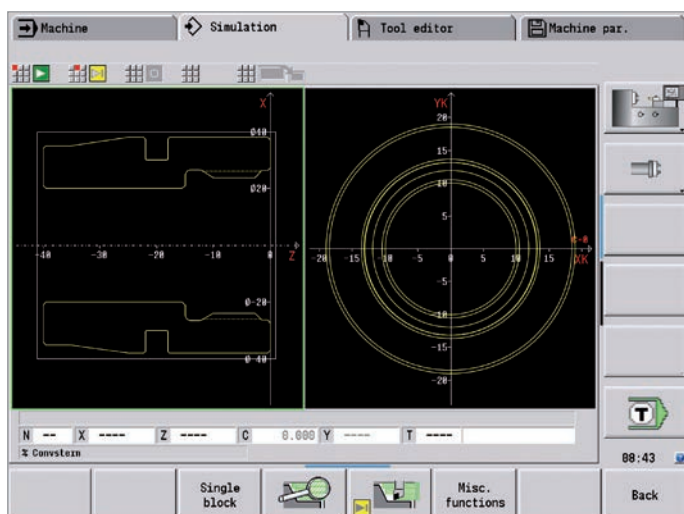
Graphic contour programming for C-axis machining (boring, drilling, and milling)
